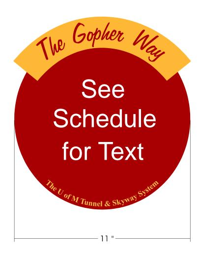
Gopherway Sign Type A and B are Fabricated from 1/8" Non-Glare Acrylic with all graphics subsurface.
